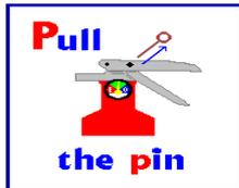
**Pull** the pin to discharge the fire extinguisher.
