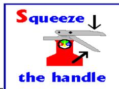
**Squeeze** the top handle or lever. This depresses a button that releases the pressurized extinguishing agent in the extinguisher.
